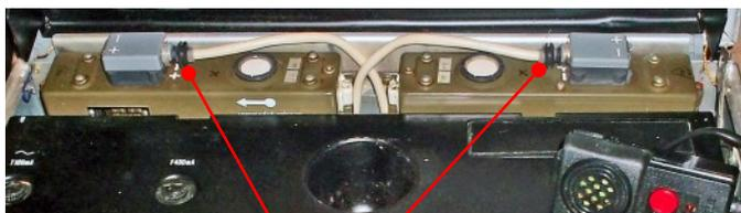
The PS-32 suitcase set was powered by two 6V NiCad batteries type QN 732 10 which were originally issued with the Czech Army type RF-10 manpack transceiver.
